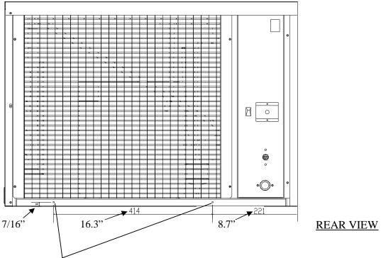
The two holes are for attachment to the ice storage bin. See drawings below.
